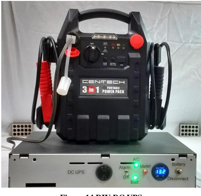
Figure 14 DIY DC UPS
