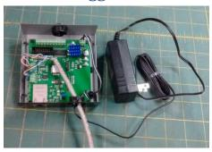
I've used a bunch of these <u>WebControl 8</u> programmable logic controllers for other home automation projects so decided to use it as the basis of the temperature logger. Unlike my other projects there is no additional electronics so I was able to use the off the shelf WebControl chassis to house the controller.
