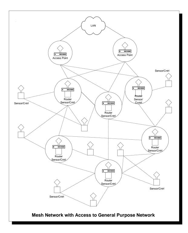
Wireless Mesh networks consist of three device classes: endpoints, routers and Access Points. Endpoints are limited functionality, often battery powered. Endpoints are able to transmit or receive messages, but do not forward external messages to other endpoints. Full function devices have all the capability of Endpoints in addition they act as routers forwarding incoming messages to the ultimate destination or the next router nearer the desired endpoint.
