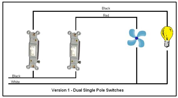
First implementation simply had two single pole (SPST) switches by each bathroom door, one for lighting other for fan. Worked for years but had to remember to turn fan on/off. Turning fan off immediately after taking a shower does not run it long enough to bring humidity down to acceptable levels.
