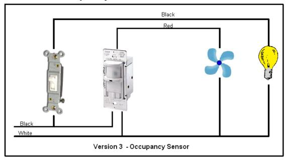
Next we tried an occupancy sensor. These are commonly used to automatically control lights in commercial buildings. Fan runs when bathroom is occupied. When sensor detects room is vacant keeps fan on for a delay period before turning it off.
