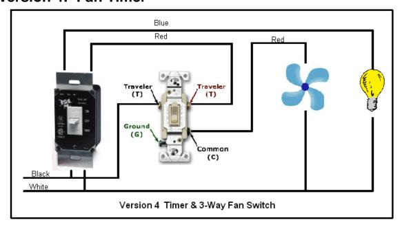
Ran across switch/timer combo designed specifically for bathroom fan control. There are several versions on the market. I chose an <u>Air King AKDT60</u>. Device costs about \$25 and fits in a single gang space.
