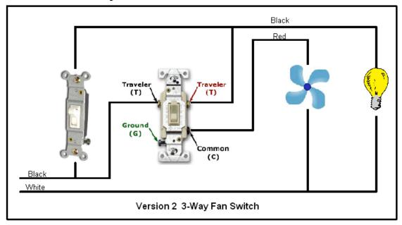
In thinking about the problem realized 3-way switch, used when two switches control a single light fixture, could automatically control fan. A 3-way switch is single pole double throw (SPDT) switch. When toggle is up common is connected to one terminal, when toggle is down common connected to other terminal.
