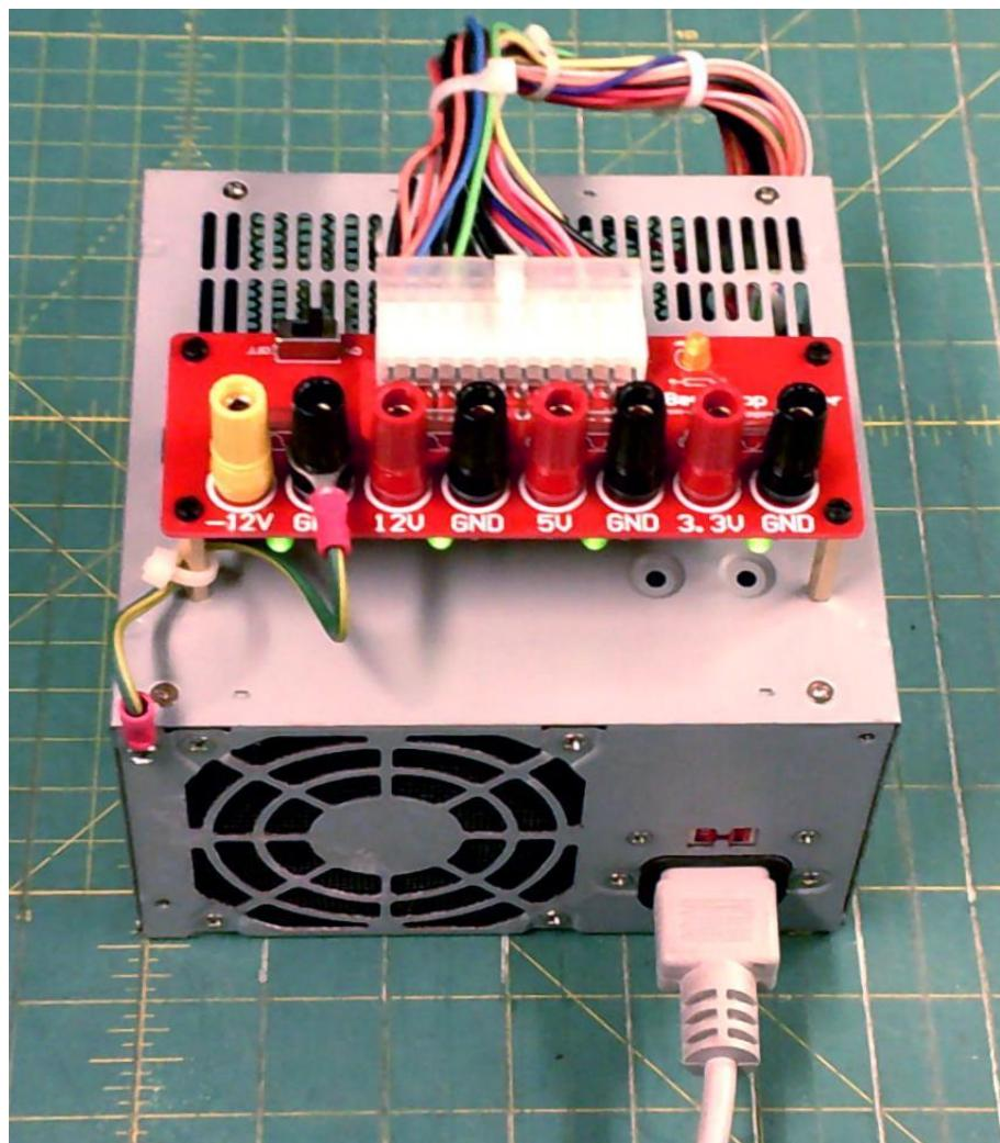
Figure 2 Finished Bench Supply
