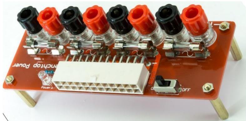
Figure 1 ATX Power Supply Breakout Board
