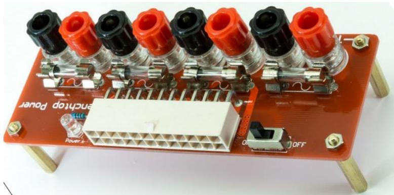
Figure 1 ATX Power Supply Breakout Board
